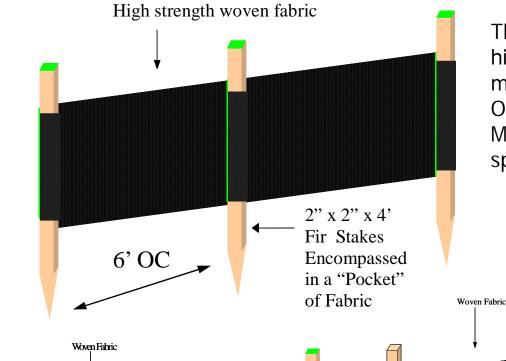
This high strength, high quality silt fence meets USA, FHA, ODOT, WSDOT, MDOT, and IDOT specifications.
