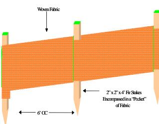
Orange Safety/Silt Fence Manage your silt and safety needs with one fence!
